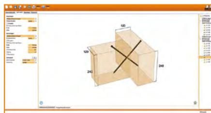
**Connection main beam/secondary beam**
