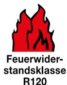
Construction products such as the MULTI-MONTI screw anchors are categorised into different fire resistance classes depending on the period for which they can resist fire. The red flame symbol and the addition "R120" show that these products are highly fire resistant and therefore proven to be able to maintain the load-bearing capacity of a mounted component (e.g. a sprinkler system) in the case of a fire for 120 minutes.
