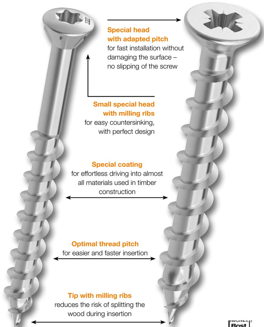
**Type:** glass strip screw, raised countersunk head with milling ribs
