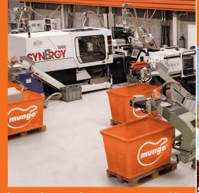
**Nylon products production, injection moulding**Mungo nylon products are made from high-grade polyamide PA6. Due to its excellent characteristics
